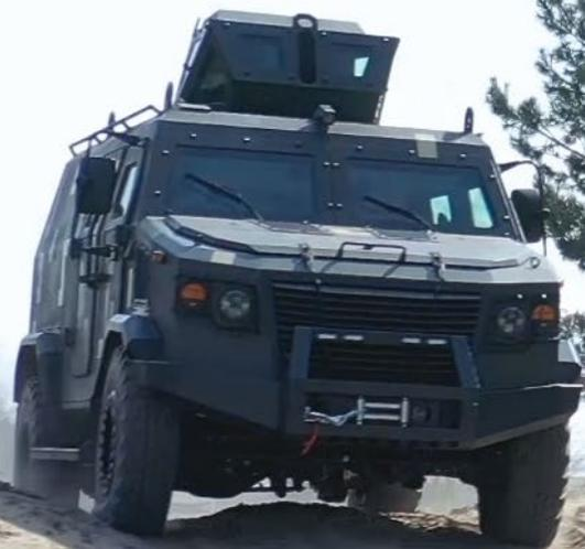
**KOZAK 5** is armored utility vehicle, intended for both tactical tasks of low intensity and for usage by police units or special operations forces. Due to small overall dimensions (the smallest among PRACTIKA armored vehicles) KOZAK-5 is perfect for actions in dense-built urban areas.
